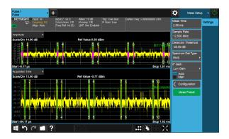
Perform pulse measurements and obtain complete results including power, time, frequency, phase and modulation with the PathWave X-Series Application.
